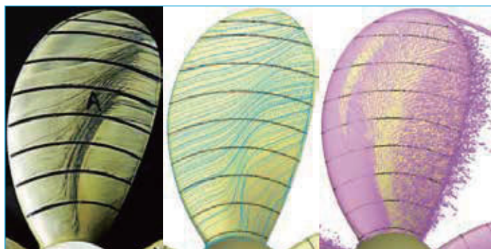
Fig.2 Flow and vortex structures on propeller surface for Reynolds number of 1.1 \times 10^6
