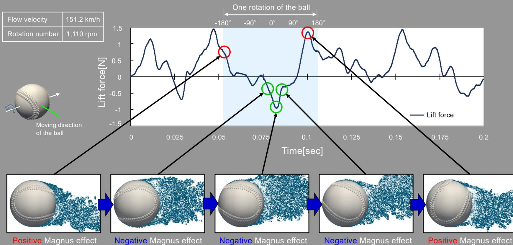
**Fig. 3 : Analysis of two-seam turbulence**
