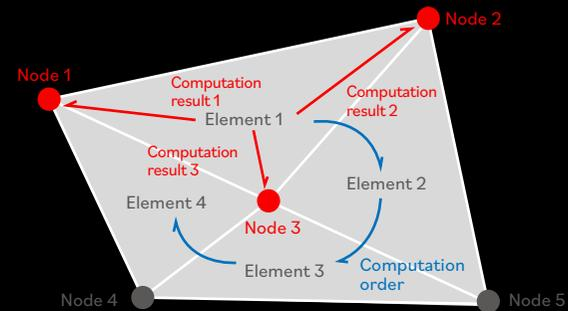
**Conventional finite element computation method**
