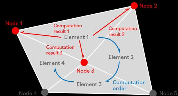
**Conventional finite element computation method**
