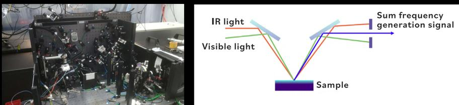
Photograph (left) and diagram (right) of the experimental setup for the sum frequency generation spectroscopy measurements. The measurements were conducted by Ohto’s collaborators at the Max Planck Institute for Polymer Research in Germany.
