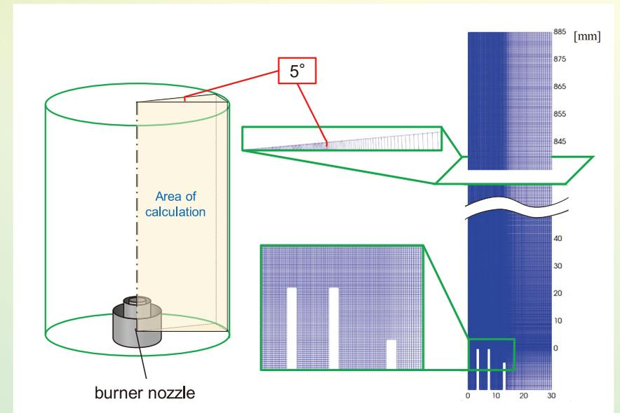
**Fig. 3 : Simulation of a laboratory-scale ammonia burner**
