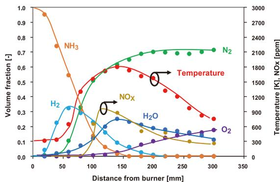
**Fig. 4 : Comparison of experiment by using ammonia burner and simulation (turbulent flow)**
