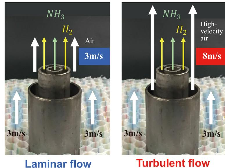
**Fig. 1 : Ammonia burner used in the research**
