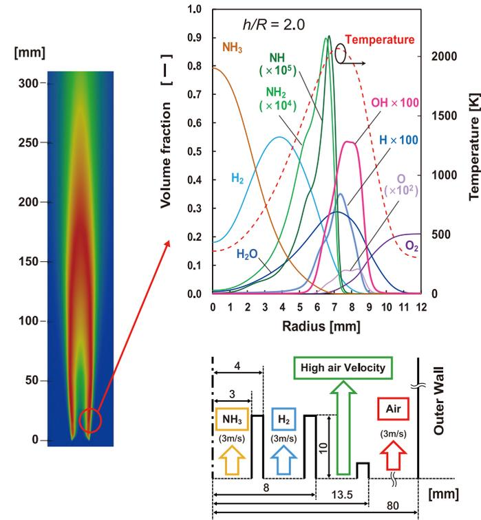
**Fig. 5 : Radical concentrations in a turbulent burner with hydrogen flame stabilizer analyzed using the supercomputer “Fugaku”**
